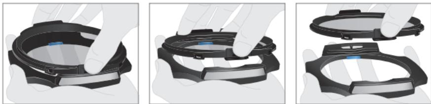
To remove the polariser (again, off camera and flat in the hand is recommended) simply push the clip hard with the ball of your thumb – on one side only – while steadying the unit with your fingers on the other clip. You do not need to squeeze both clips.
