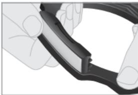
Place the appropriate size of grey cover plate into the open side, making sure it is in the correct orientation, to complete the assembly. Keep all the spare parts somewhere safe, as you will need them should you wish to reconfigure the holder at a later date.
