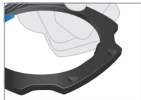
Insert the larger, flat end of the removal tool into the small slot in the middle of the base of the guide block. Push the tool in until you feel resistance. You are not prising the block loose – you are releasing a catch under the block, which holds it in place.
