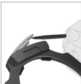
Use the narrow end of the removal tool to pick out the grey cover plate. The cover plates vary in size, according to whether the filter guide block has one, two or three slots. Keep the plates safe with the blocks for future use.
