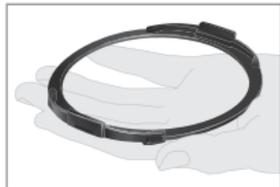
The easiest way to fit the polariser is to start off with the ring flat in your hand. Make sure the two finger grips on either side are pointing upwards.
